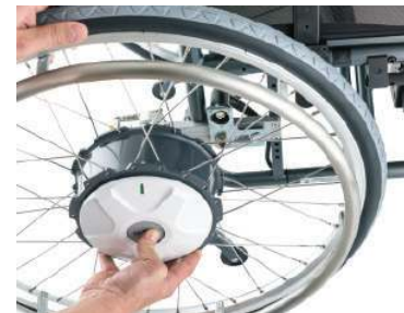
Use the quick-release mechanism to remove the drive wheels
